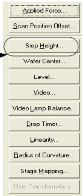
12. **Range:** Choose the range to be calibrated. Select the appropriate step height standard for use in calibrating the selected range. (See the circled area in *Figure 12.11*.)
