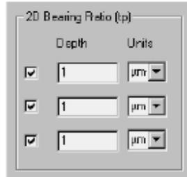
2. The depth is set down from the highest peak in the scan. It can be set in either microns (µm) or angstroms (Å). Determine which units are going to be used and, if a change is necessary, click the menu arrow under units to display its menu.
