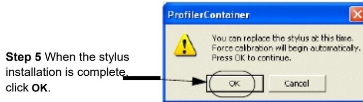
6. The system performs an Applied Force calibration.
