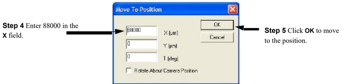
5. After the entry is complete, click **OK** to close the dialog box and position the stylus at the new coordinates. (See *Figure 12.19*.)
