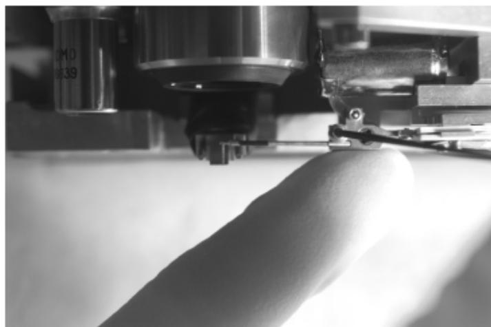
12. With the stylus clamp screw loose, take hold of the stylus with tweezers and pull gently straight to the left until the stylus comes free. (See *Figure 14.8*.)
