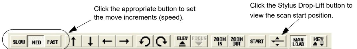
3. Click the **Stylus Drop-Lift** button to null the stylus on the sample and confirm the scan position.
