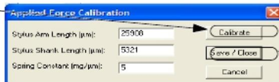
**Step 4** When the calibration is complete, click **Save/Close** to save the calibration results of the Applied Force Calibration.
