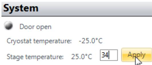
On the right bottom side of the Acquisition software there is a System window which gives you information about the door and temperature state.
