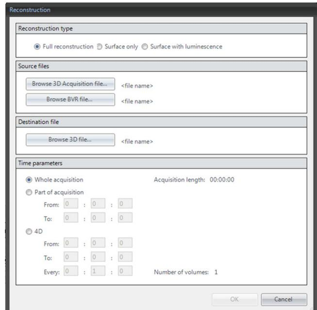
As the reconstruction may take time and CPU resources, you can postpone the process and plan a task schedule by selecting reconstruct later and entering the time of execution. Then press on start reconstruction.
