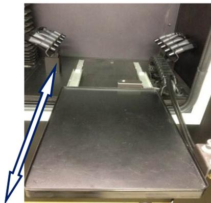
A set of black walls is available for optical isolation of animals. This may help avoiding false measurements due to lighting of an animal by another, and should be used when several animals are imaged simultaneously.
