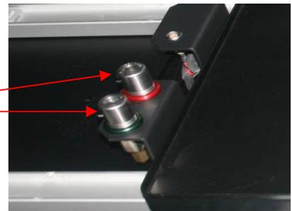
The anesthesia bar includes 5 "T taps", each corresponding to a mouse position. The T taps of the anesthesia bar should be rotated so that the selected cones are provided with gas as desired. Each T tap can allow to:
