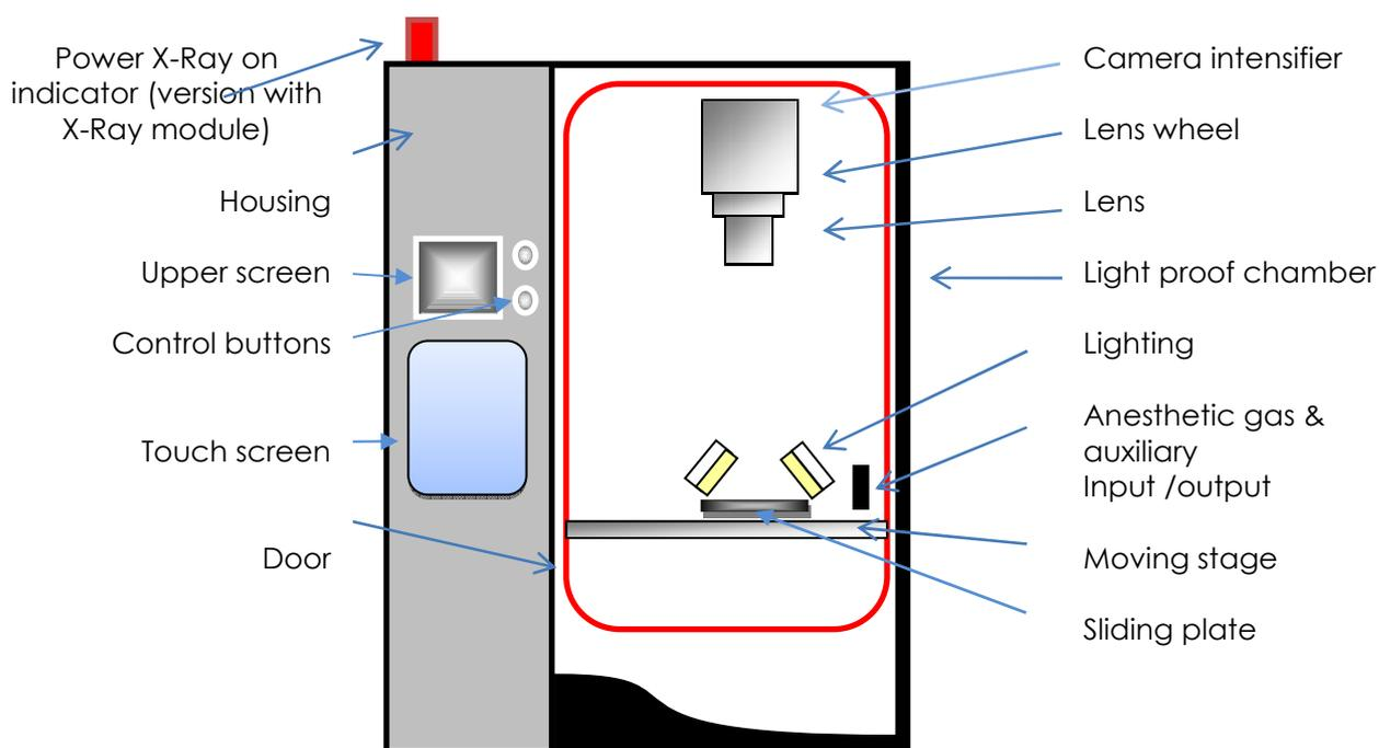
The detection system of the equipment is made of:
