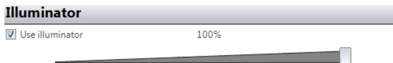
**NOTE : Strong illumination settings can damage the detector. Illuminator power must be increased progressively.**
