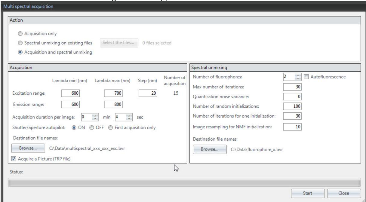
In the right Spectral unmixing window define the number of fluorophores you are going to image.
