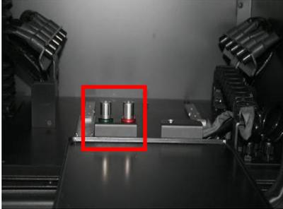
gas connectors inside the chamber
