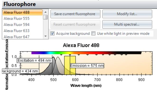
The optical parameters window in fluorescence integration mode
